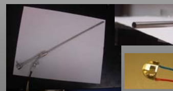
MEMS-based Endoscope fits into a standard Cystoscope
