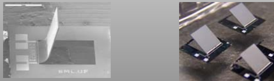
Scanning Range: >120°, among the largest ever reported Driving Voltage: <20V, lowest among devices with similar scanning range Aperture Size: 1mm
